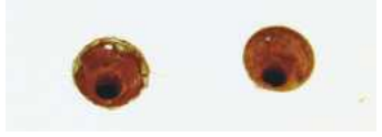
▲ With the screws removed the Optimaxx hole on the right shows a clean countersink
